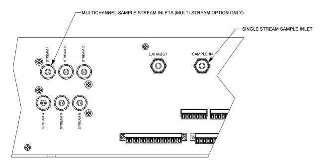
Figure 4-2: Pneumatic Connections, Rack Mount Configuration
